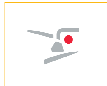
The safety sensor stops the movement of the chair when the chair is deflected.
