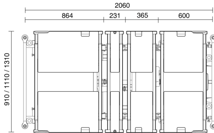
Figure 5.1: Mattress platform dimensions Olympia Bariatric bed
